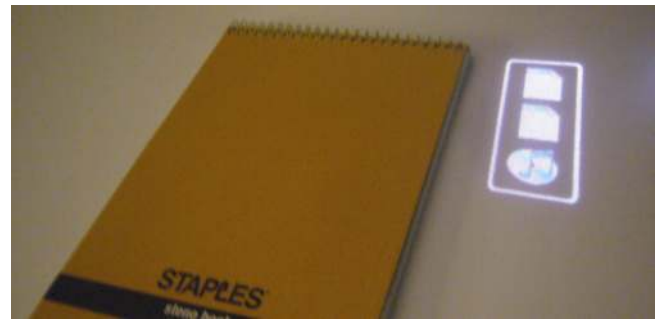
Figure 6. Physical bookmarks for digital tasks. When the notebook is detected on the table, Bonfire projects a list of applications that were open when the notebook was last seen.
