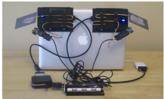
Figure 2. Rear view of the Bonfire prototype hardware setup. Projectors and cameras are mounted on the laptop screen and connected via a USB hub. Mirrors reflect the projected images to the sides of the keyboard.
