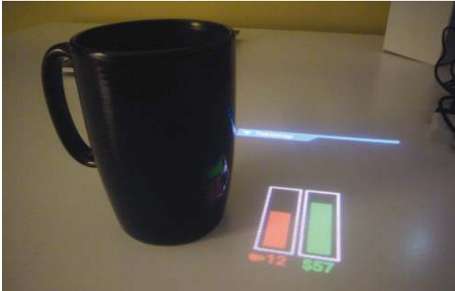
Figure 5. Augmenting interaction with physical objects. After the coffee cup is detected, Bonfire projects a graph of cups of coffee consumed and an approximate cost this week. When the user taps the graph, a detailed view is shown on the laptop screen.
