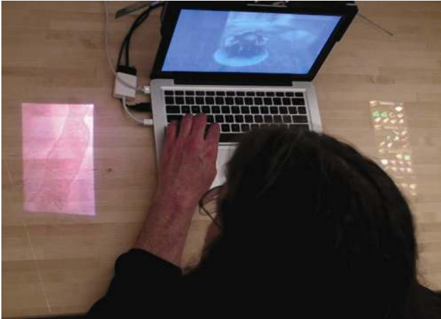
Figure 10. Enhancing MMORPG game play. The laptop screen is used for 3D world navigation and player-to-player communication. Map view and player inventory are shown in the projection areas.
