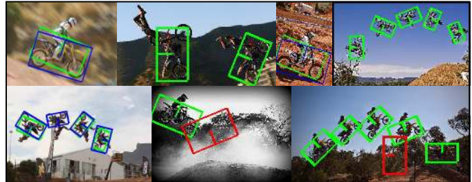
Fig. 13: Cascaded BRFs for rotation invariant object detection. Green rectangles are true positives, while red ones are false positives. Blue rectangles are ground truth.
