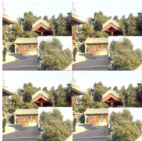
Figure 1. Examples of high-frequency recovery. These visual cases are compressed frame (top left), prediction of STDF (top right), prediction of a model trained with L1 + FFT loss (ours) (bottom left), and the ground truth (bottom right).
