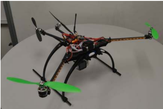
Figure 6: VTail quadcopter: Bird view
