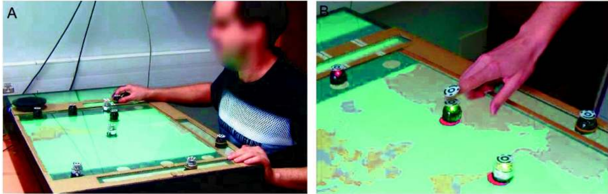
Fig. 1. (A) BotMap is composed of an interactive tabletop and several robots, tracked by a camera. Each robot represents a landmark and moves to its new position whenever the map is refreshed. On the picture, a blind user is zooming with the Sliders interface. (B) Users can select a robot to retrieve the name of the corresponding landmark.
