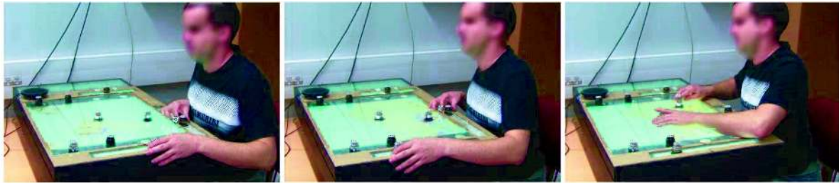
Fig. 4. Panning with the sliders interface: A participant moves the two sliders for panning (left and middle) and explores the map once the robots are in place (right).
