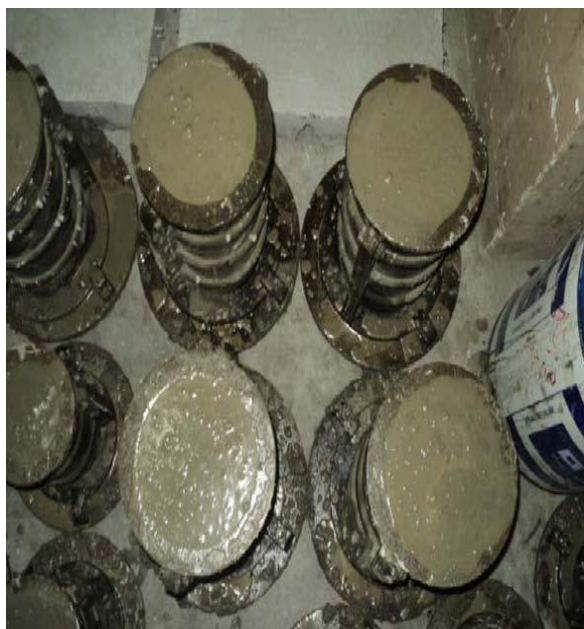
Figure 2. Casting cylinders of 100mm diameter, depth 200mm size.
