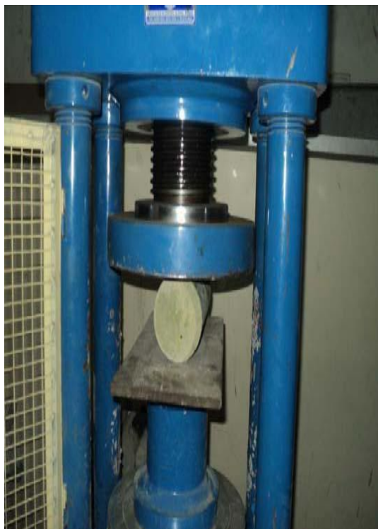
Figure 4. Testing of cylinder in compression testing machine after 28days curing.
