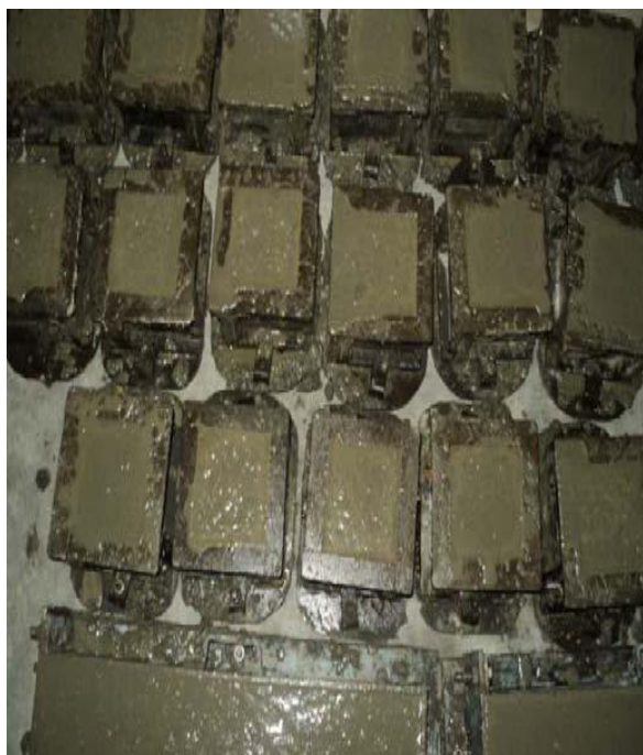
Figure 1. Casting cubes of 100 X 100 X 100mm size.
