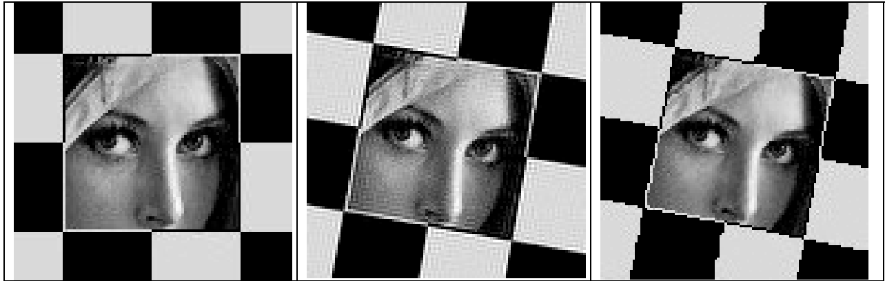
Fig. 11. Image (upper) rotation with sliding window non-adaptive (left) and adaptive DCT sinc-interpolation (right). Note disappearance of oscillations at sharp edges thanks to switching between sinc-interpolation and nearest neighbor interpolation at the boundaries of black and white squares
