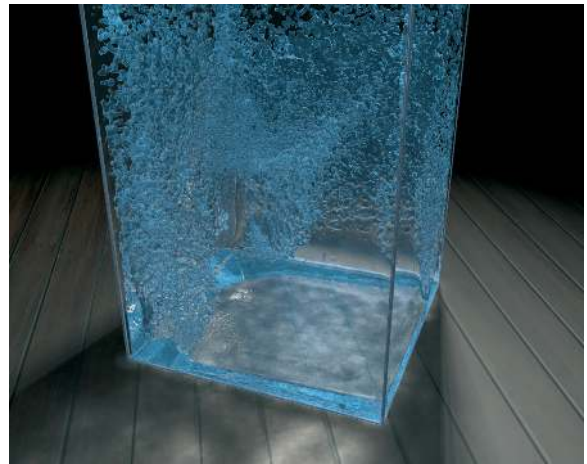
Figure 6: CBD large scene. A corner breaking dam with 1.7 million particles. Overall computation time 16.5 hours for 20 real seconds, \Delta t_{min} = 1.7 \cdot 10^{-4} , \Delta t_{max} = 1.66 \cdot 10^{-3} .
