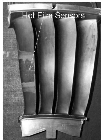
Figure 4 NGV2 of the BR715UHL LP turbine showing the hot film array of sensors on the right hand aerofoil.
