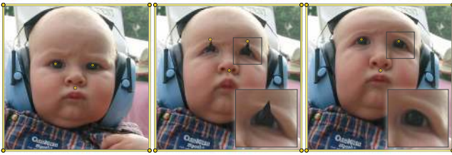
Figure 9: Weights must be smooth everywhere, especially at internal handles, which are likely to correspond to important features. Weights that have discontinuities at handles, like Harmonic Coordinates (center), introduce tearing artifacts with even slight changes in the handles. Our weights are smooth, as shown on the right.
