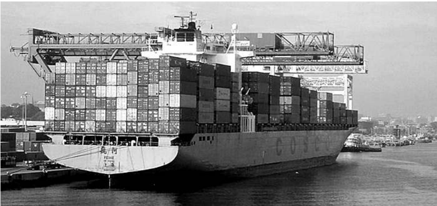
Above: The 1994-built container ship Feihe , operated by state-owned China Overseas Shipping Company (COSCO), has a capacity of 4,315 TEUs. Containers are stacked thirteen across as the ship is unloaded at the port of Boston. Below: Efficiency requires that refrigeration equipment not protrude beyond the dimensions of a container. Eimskip is a small Scandinavian company that specializes in service to Iceland.
