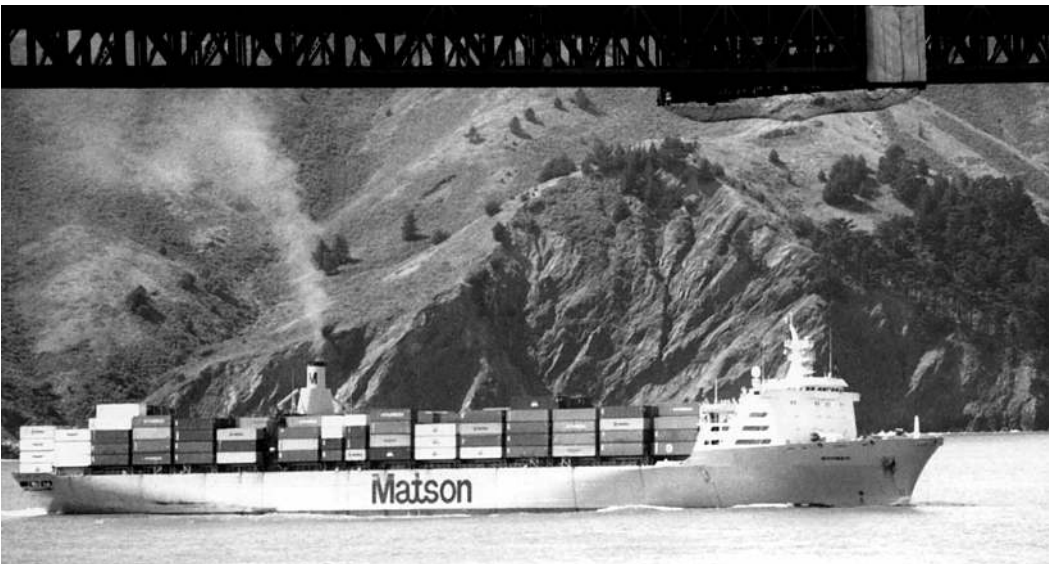
With a forward deck house and machinery slightly abaft of midships, Matson's Mahimahi steams under the Golden Gate Bridge into San Francisco Harbor. The general design recalls Sea-Land's famous SL-7. (Paul Tully)
