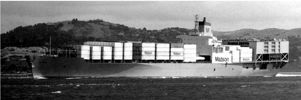
Originally a ro/ro vessel, Matsonia was later converted into an unusual hybrid. Forward of the deck house are conventional container cells, but abaft is a garage for transporting automobiles between Hawaii and the mainland. (Paul Tully)
