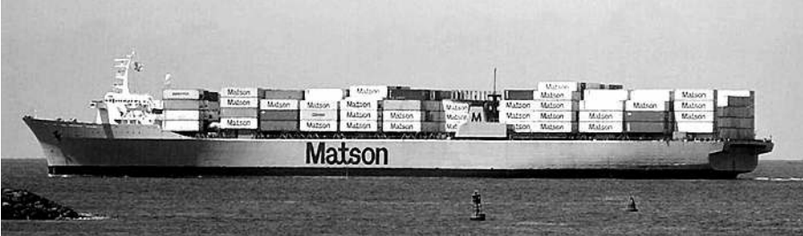
Lihue is currently a cellular container ship in the Matson fleet, but began life as a LASH-type cargo vessel owned by Pacific Far East Line. (Roger J. Cudahy)
