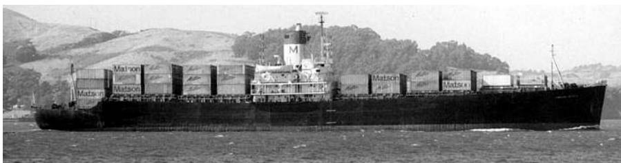
Above: Matson's Hawaiian Citizen began life as the C-3 cargo ship Sea Wren and was converted into a container ship in 1960. (Paul Tully). Below: Matson's Kauai , shown after conversion into a hatchcoverless container ship. (Paul Tully)
