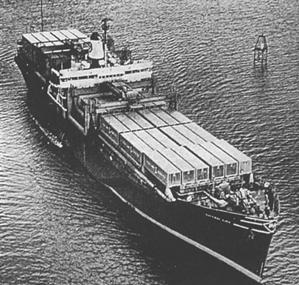
The converted C-2 cargo ship Gateway City carried containers both on deck and in below-deck cells.
