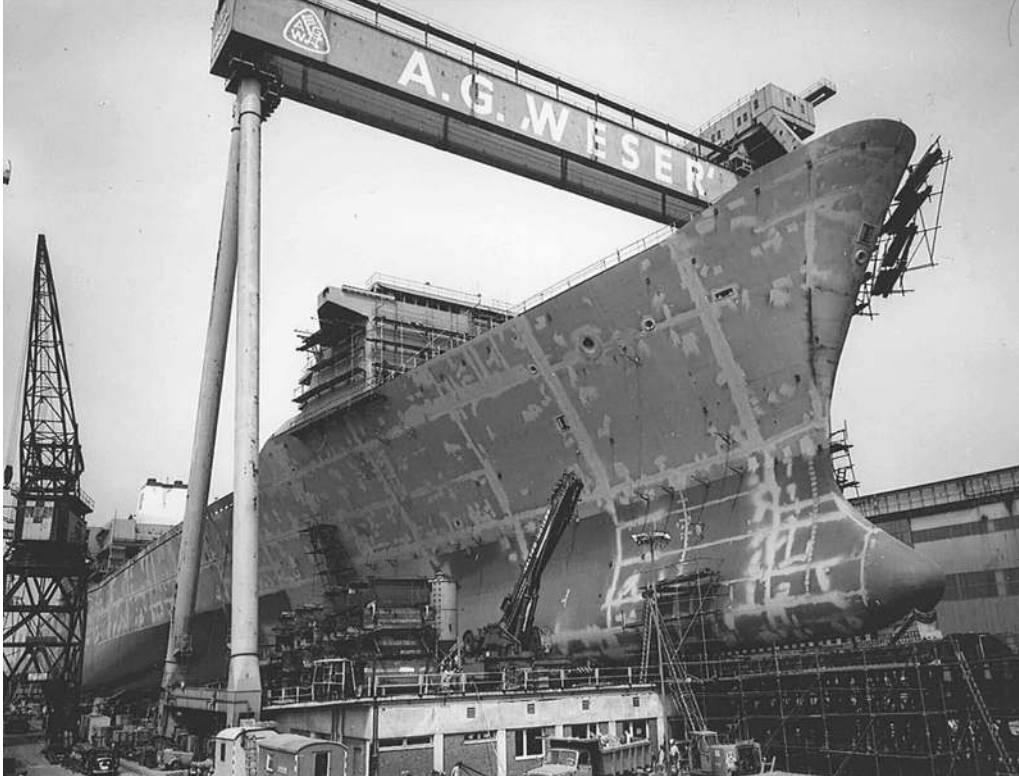
A thin, knife-like bow was a critical design feature to ensure that Sea-Land's SL-7 would achieve high-speed performance. (McLean Foundation)
