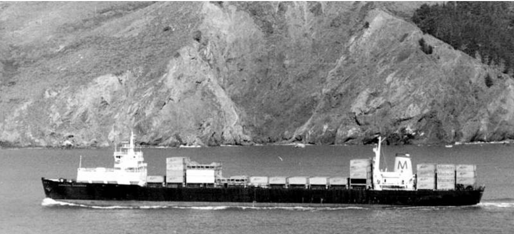
Like many of Sea-Land's early container ships, Matson Navigation Company's Hawaiian Monarch was once a C-4 cargo ship. (Thompson Tully)
