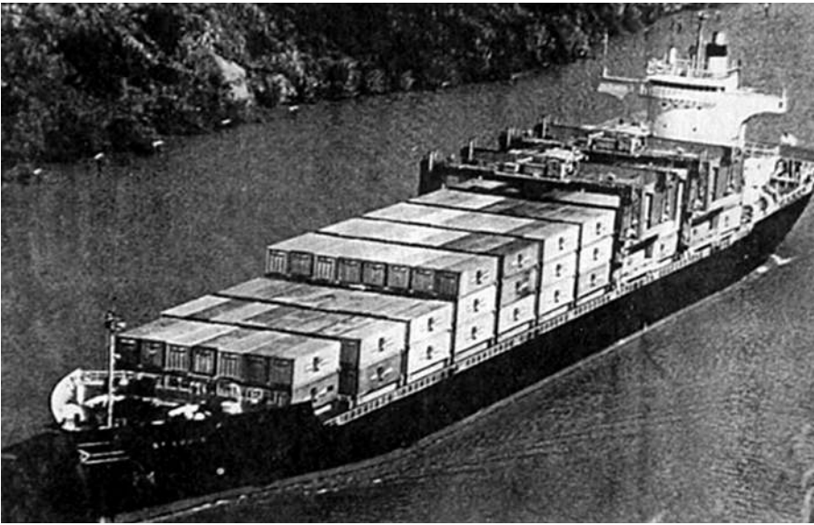
Sea-Land's St. Louis was converted into a cellular container ship from the C-4 troop transport General M. L. Hersey .
