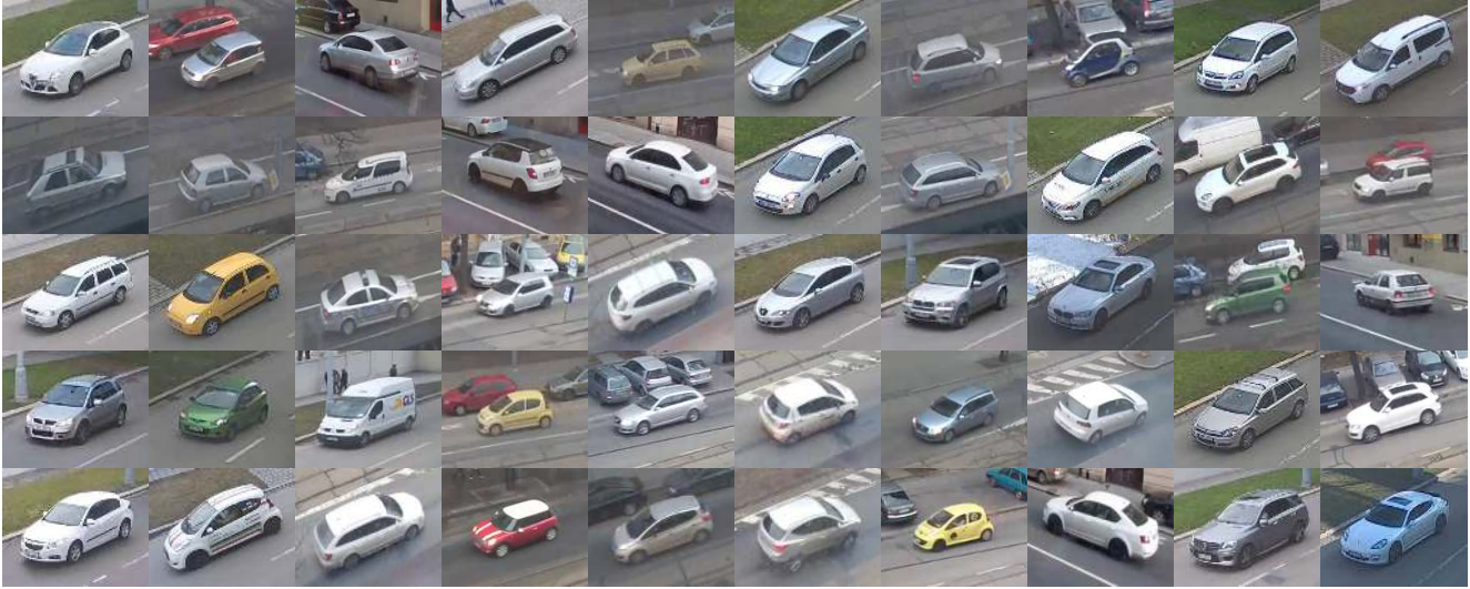
Figure 7. A sample of the novel BoxCars dataset. In total, it captures 21,250 vehicles in 63,750 images, from 27 different makes (148 fine-grained classes).
