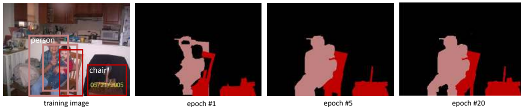
Figure 3: Update of segmentation masks during training. Here we show the masks in epoch #1, epoch #5, and epoch #20. Each segmentation mask will be used as the supervision for the next epoch.
