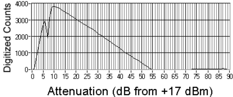
Figure 3. Degraded Dynamic Range – about 45 dB
