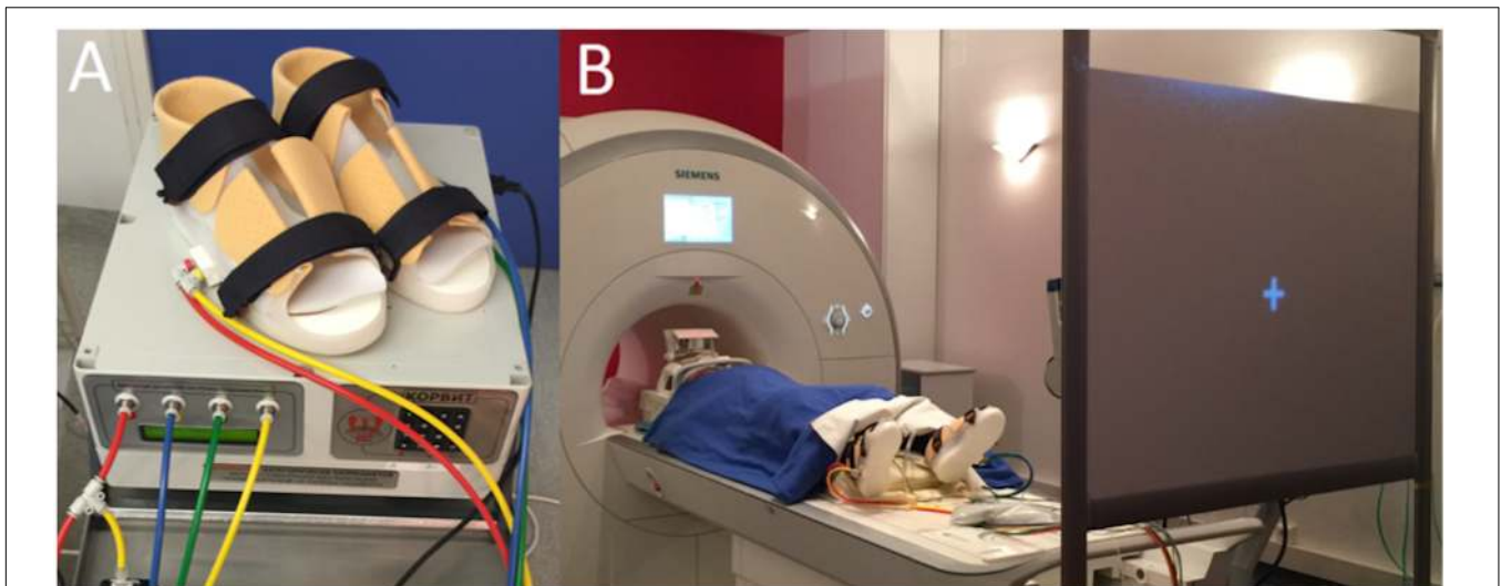
FIGURE 1 | (A) Korvit MRI-compatible simulator, composed of a control unit, air ducts and pneumatic boots. (B) Participant lying in the scanner and wearing the Korvit boots, looking at a screen through a prism.
