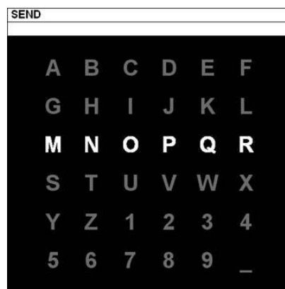
Fig. 7. Typical panel displayed on the monitor screen of a BCI system based on the P300 potential [21].
