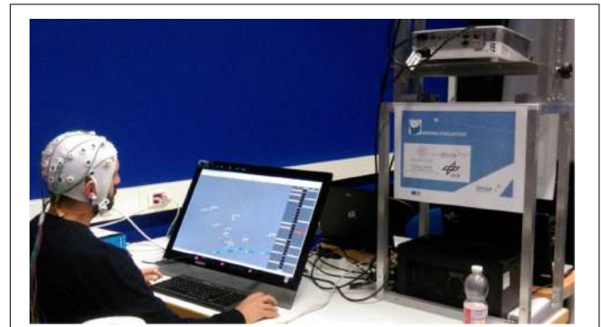
FIGURE 1 | The figure shows a moment of the experimental task. The ATCo is supervising a traffic situation over the ATM interface.
