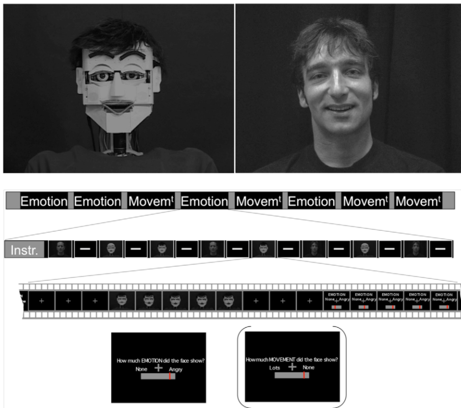
Figure 1. Experimental paradigm. Top: single frame from a Human (left) and Robot (right) Joy stimulus. Middle: organization of an fMRI recording session, showing first, the randomization of the order of the rating blocks (Emotion and Movement) within an acquisition run, then the organization a block starting with a reminder of the instruction (Instr.), and finally the presentation of one stimulus followed by the response screen. Bottom: response screen used in the emotion task (and the motion task between parentheses). doi:10.1371/journal.pone.0011577.g001
