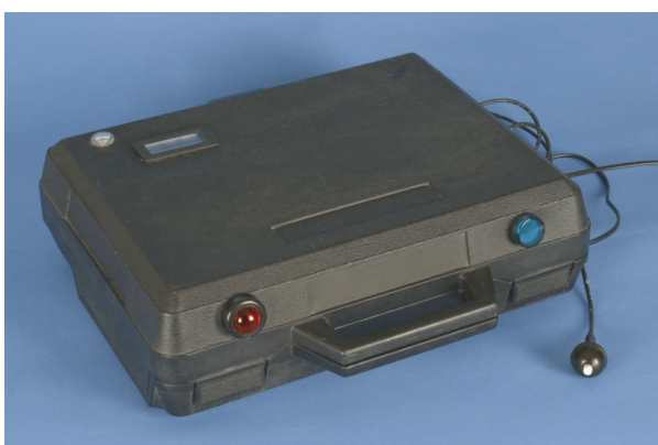
Figure 3 The external suitcase containing the logic gate electronics, the trigger, the green and red lamp, and the clock.
