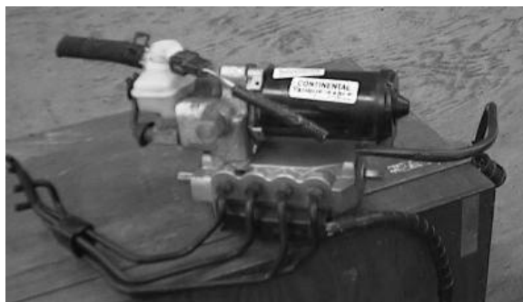
Figure 4.24: Photograph of the Red Lincoln Towncar’s ABS unit
