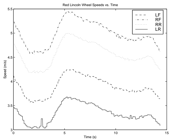
Figure 4.23: Speed measurements from each of the Red Lincoln’s four wheels as the car turns circles to the left.
