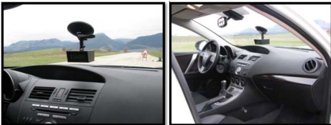
Figure 7. Location of XL Meter™ Pro in the vehicle
