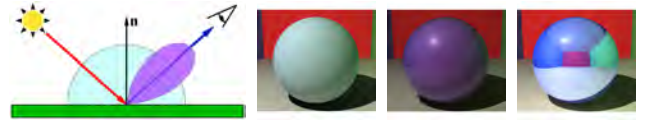
(a) Basic reflection models (b) Diffuse (c) Glossy (d) Specular Figure 4: (a) Basic reflectance models of the incoming light (in red): perfect diffuse (light blue), glossy (purple) and perfect specular (blue). In (b-d) renderings of diffuse, glossy and specular spheres are shown, placed inside a Cornell box [GTGB84].
