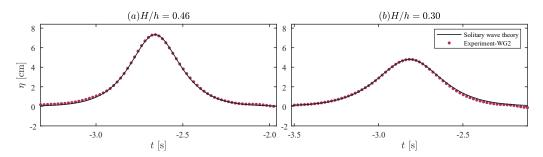
**Figure 3.** Comparison in terms of a wave-profile time series between ensemble-averaged measurements at WG2 and the third order theoretical solution of solitary waves [29] for the cases of (**a**) H/h = 0.46 and (**b**) H/h = 0.30.
