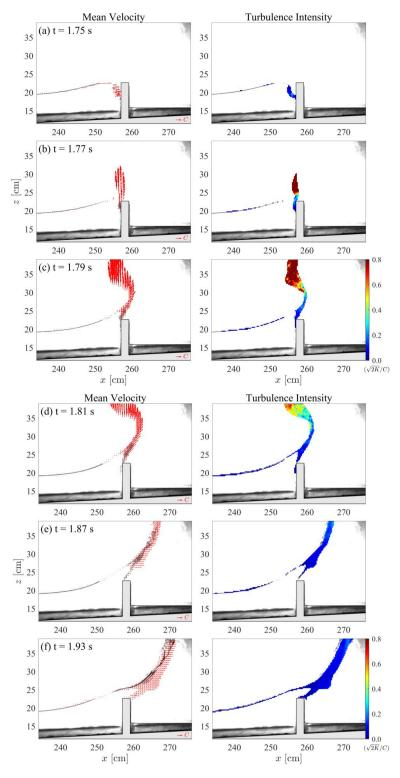
**Figure 9.** Ensemble-averaged velocity fields (left column) and normalized turbulence intensity (right column) superimposed with instantaneous background images, for the case of H/h = 0.30, at (**a**) t = 1.75 s, (**b**) t = 1.77 s, (**c**) t = 1.79 s, (**d**) t = 1.81 s, (**e**) t = 1.87 s, and (**f**) t = 1.93 s.
