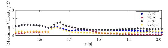
**Figure 7.** Time history of maximum fluid velocities and turbulence intensities normalized by the wave celerity, *C*, for the case of H/h = 0.46.
