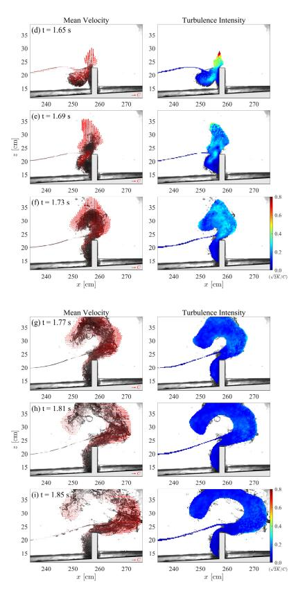
**Figure 5.** Ensemble-averaged velocity fields (left column) and normalized turbulence intensity (right column) superimposed with instantaneous background images, for the case of H/h = 0.46, at (a) t = 1.53 s, (b) t =1.57 s, (c) t = 1.61 s, (d) t = 1.65 s, (e) t = 1.69 s, (f) t = 1.73 s, (g) t = 1.77 s, (h) t = 1.81 s, and (i) t = 1.85 s.
