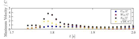
**Figure 10.** Time history of maximum fluid velocities and turbulence intensities normalized by the wave celerity, *C*, for the case of H/h = 0.30.
