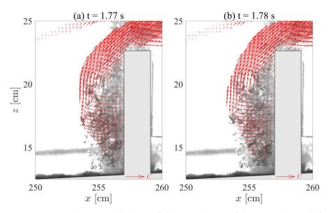
**Figure 6.** Ensemble-averaged velocity fields near the toe of the vertical seawall for the case of H/h = 0.46 at (a) t = 1.77 s and (b) t = 1.78 s.
