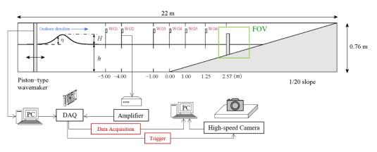
Figure 2. Sketch of experimental setup and instruments used in this study (not to scale).
