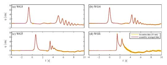
**Figure 4.** Measured time history of free surface elevations at the four locations, for the case of H/h = 0.46.
