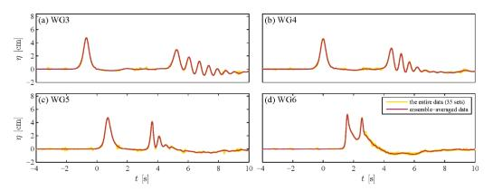
**Figure 8.** Measured time history of free surface elevations at the four locations, for the case of H/h = 0.30.
