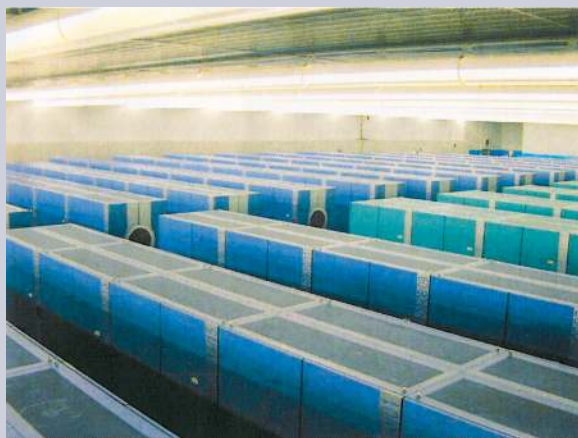
FIG. SB1. The Earth Simulator machine of the Frontier Research Project. The machine is located in Yokohama, Japan. Its measured performance is 35.61 Tflops. It consists of 640 nodes that are connected by a high-speed network. Each node contains eight vector processors with 16 GB of memory, for a total of 5120 processors and 10 TB of memory. The Earth Simulator is capable of running a super-GCM fast enough to enable practical climate change simulations.
