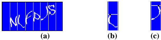
Fig 12. Recognising ‘L’ and ‘J’. (a) A segmented challenge. (b) The 2 nd segment was normalised and successfully recognised as ‘L’. (c) The 5 th segment was normalised and successfully recognised as ‘J’.
