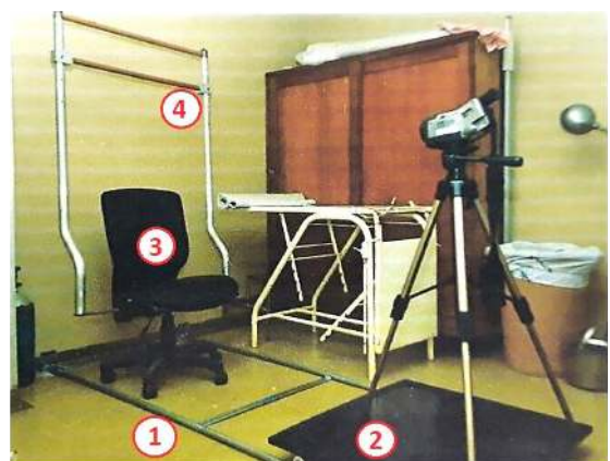
Figure 2. Mechanical device to place patient in the right position during images acquisition. (1) the trails used to move the camera support car, there are two (2) of them and they are placed on the floor; (2) plate-shaped car to support camera's tripod; (3) swivel chair where the patient is placed on; (4) arms support, which consists of a horizontal bar that moves vertically so the patient can put the hands up during the exam.
