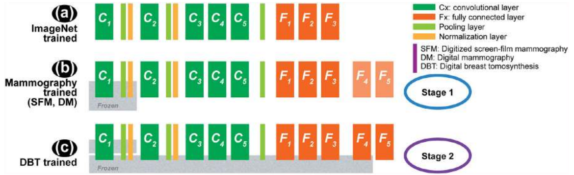
Fig. 1. Overview of the CNN structures used in the multi-stage transfer learning. (a) ImageNet trained CNN with five convolutional layers and four fully connected layers. (b) Stage 1 transfer learning using mammography data. Two fully connected layers ( F_4 and F_5 ) are added to the ImageNet structure in (a). (c) Stage 2 transfer learning using DBT data. Note that (b) and (c) show three strategies of fine-tuning by freezing the CNN at different layers. The choice of fine-tuning layers is explained in sections II-C and II-D.
