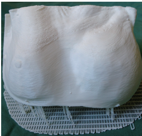
Figure 2 3D printed haptic model of the breasts in Figure 1 using Cube 2 printer (3D Systems, Rock Hill, SC, USA) and polylactic acid (PLA) filaments. Reproduced with permission from Chae et al. (76).
