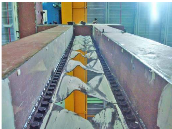
Fig. 7. SPSL's yielding at 1.6% drift
