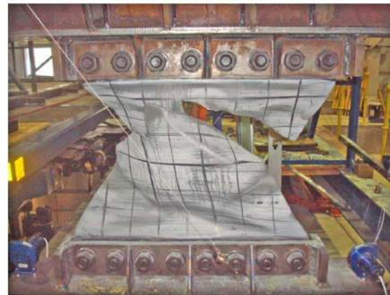
Fig. 14. (a) Link shear versus total rotation hysteretic curve for unrestrained specimen; (b) link condition after testing
