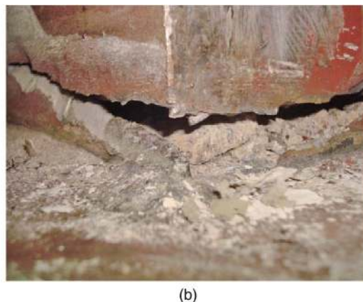
Fig. 8. (a) Local buckling of west column 2.2% drift; (b) fracture at 2.7% drift
