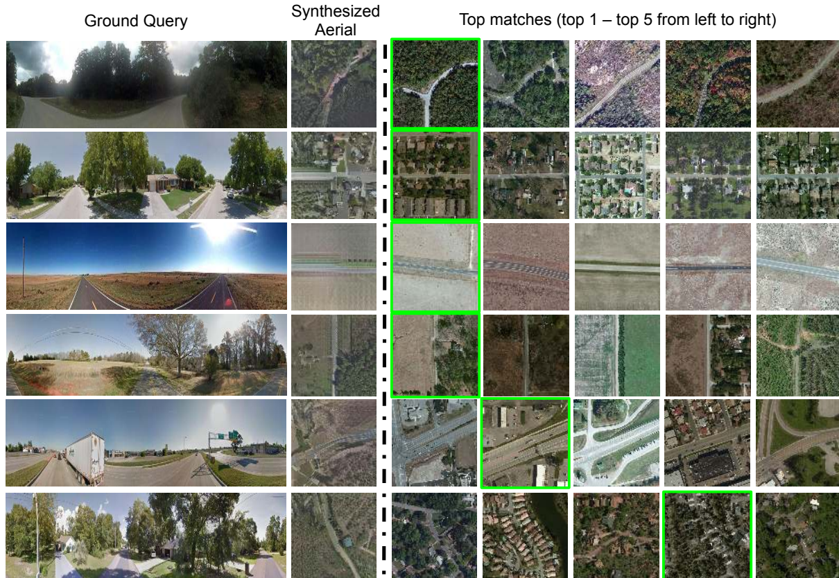
Figure 3: Image retrieval examples on CVUSA dataset [45]. For each query ground-level panorama, the synthesized aerial image is shown alongside, followed by the five closest aerial images retrieved by proposed Feature Fusion method. The correct matching (ground truth) aerial images are shown in green boxes. Rows 5 and 6 show examples where the ground truth aerial images are retrieved at the second and fourth positions respectively.
