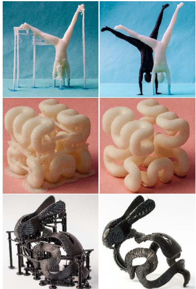
Figure 16: Models printed with our technique, scaffoldings on the left and cleanup model on the right. Top: The Gymnast model. Middle: The curved Hilbert cube model. Bottom: The 5cm Bunny Peel model. Hilbert cube model: thingiverse.com/thing:16343 by tbuser . Bunny peel model: thingiverse.com/thing:131054 by user meshmixer .
