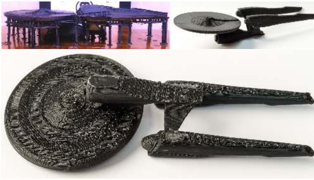
Figure 9: Top: Printout of the Enterprise model. Bottom: Underside after cleanup. We broke the engine connectors during cleanup and had to glue them back (only case where glue was involved). Print time: 3h14, 9.89m of filament.
