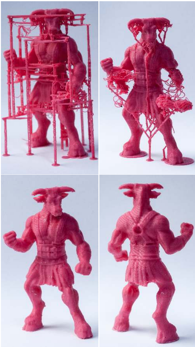
Figure 17: Top left: The Minotaur printed with our technique. Print time: 2h37m, 7.66m of filament. Top right: Attempt at printing the MeshMixer version. Print time (same parameters): 2h04, 6.7m of plastic. We also had to add a raft below each feet. On our model, the stability analysis automatically added a raft beneath each feet (visible in picture). Bottom: Model printed with our technique after clean up, front and back.
