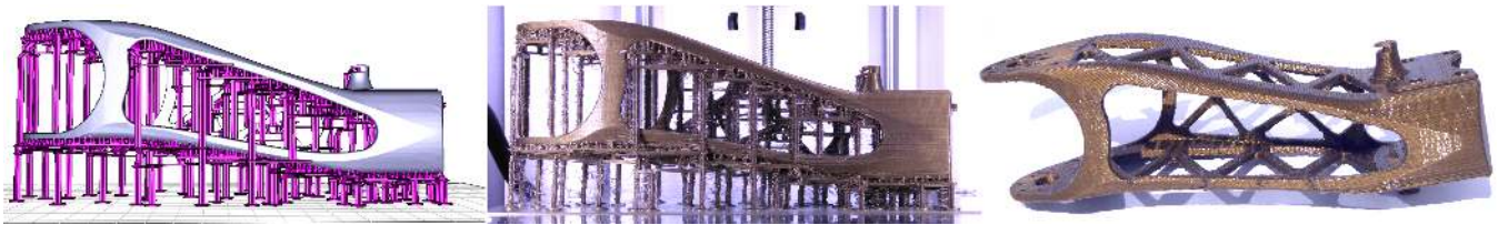
Figure 1: The upper leg of the Poppy robot ( www.poppy-project.org ) cannot be 3D printed on low cost FDM printers without support. Our technique automatically generates scaffoldings made of horizontal bridges supported by vertical pillars, shown in purple. The print is shown in the middle and on the right after clean up. Bridges are strong and stable, increasing the print reliability while having a low material usage.
