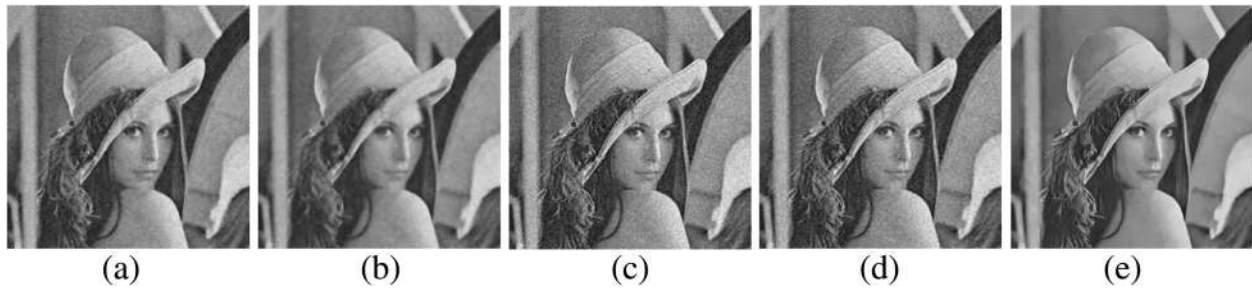
Fig. 2 Visual comparisons of denoising results on Lena image corrupted by additive white Gaussian noise with standard deviation 30: a Wiener filtering [16] (PSNR = 27.81 dB; SSIM = 0.707); b Bilateral filtering [10] (PSNR = 27.88 dB; SSIM = 0.712); c PCA method [87] (PSNR = 26.68 dB; SSIM = 0.596); d Wavelet transform domain method [89] (PSNR = 21.74 dB; SSIM = 0.316); e Collaborative filtering: BM3D [55] (PSNR = 31.26 dB; SSIM = 0.845)
