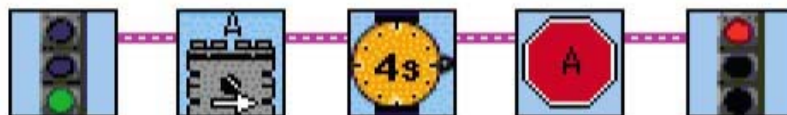
Figure 3: A basic Inventor program that turns on motor A, waits for 4 seconds, and turns off motor A.
