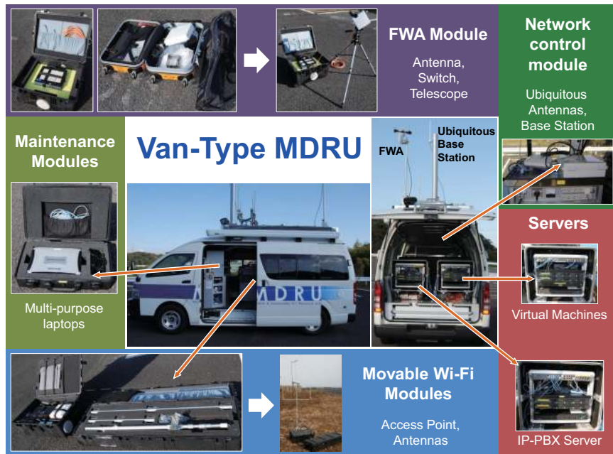
Fig. 3. Modules inside the van-type MDRU.
