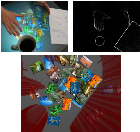
Figure 5. Top left: Particle proxies approximate the shape of multiple contacts and physical objects (cup, notepad). Top right: Sobel image shows contact contours. Bottom: Particles (red) as they project into the 3D scene.
