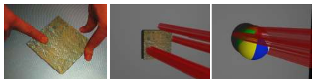
Figure 4. Particle proxies approximate the shape of multiple contacts. Left: applying friction from the top, and collision from the side to grip a block. Middle: Long proxy particle objects (red) illustrated. Right: Particle proxies accommodate non-flat objects. Here we model each proxy as a long capsule.
