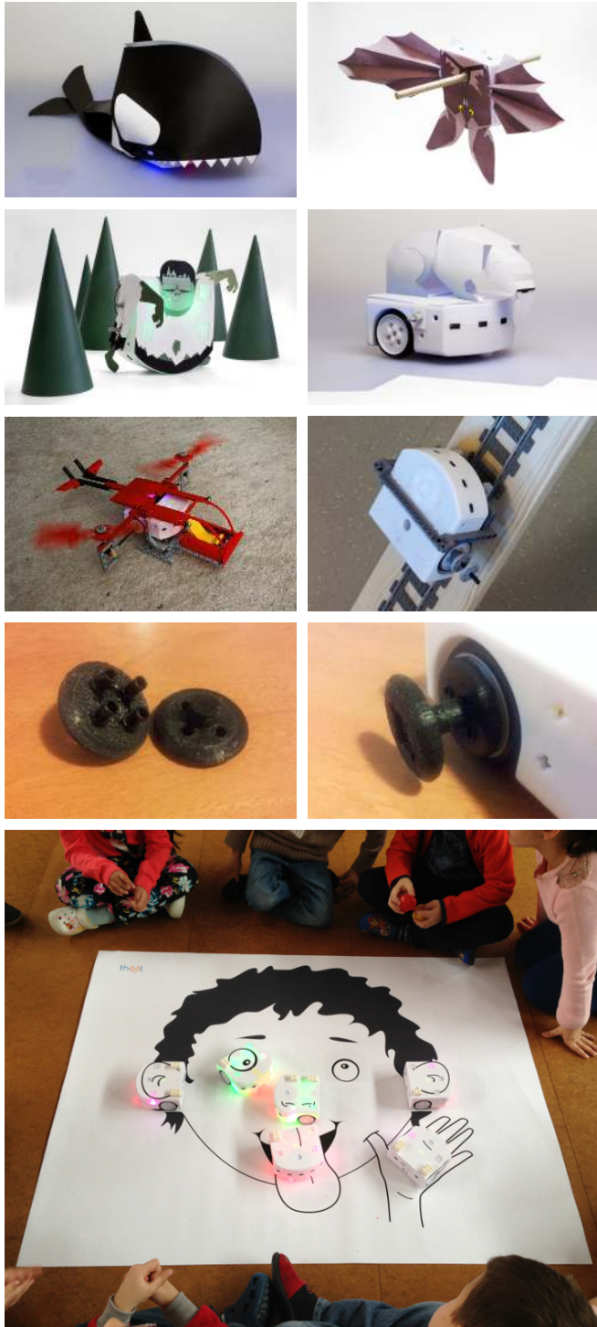
Fig. 2: Examples of extensions of the Thymio basic robot with paper or cardboard body extensions (top four images), using LEGO® structural extensions (third row), using 3D-printed extensions (fourth row) or using a printed environment (bottom).
