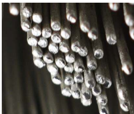
Figure 2. Macro-photograph showing the way the coating on the tips of the bristles is wearing out after months of use. The tips looking dark in this photography are no longer properly coated.
