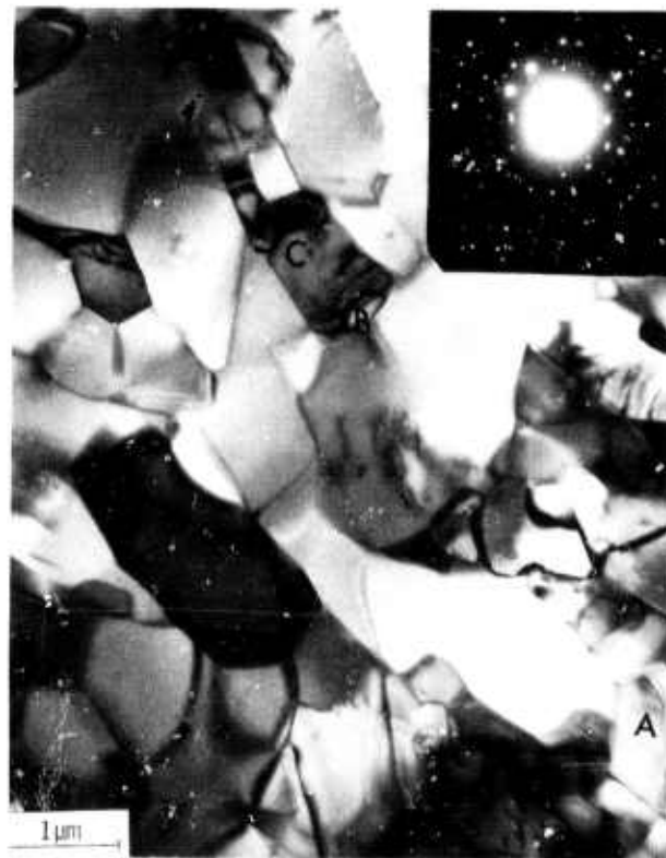
Figure 5.24 — Transmission micrograph (100 kV) showing general grain morphology of hot pressed Si 3 N 4 . Note the absence of a ring pattern, indicating non-random grain orientations
