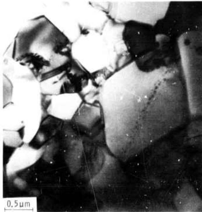
Figure 5.25 — Chain of impurities across a grain occasionally observed in transmission microscopy. (100 kV)
