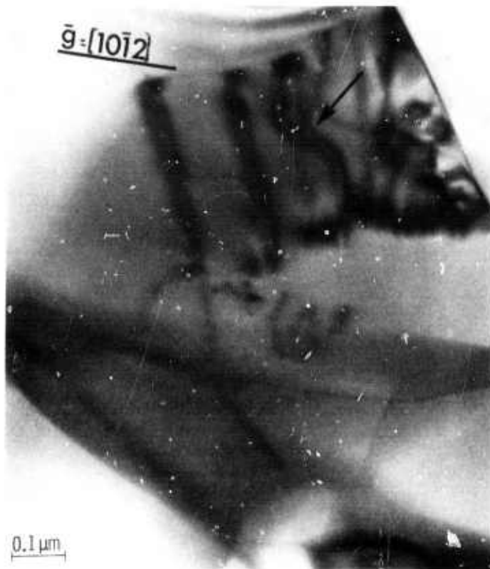
Figure 5.31 — Near dipoles (arrow) in an \alpha grain \bar{g} = [10\bar{1}2] , [\bar{1}3\bar{2}2] ZA (100kV)
