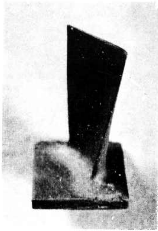
Figure 3.18 — Turbine Rotor Blade Made From CVD Silicon Carbide (Courtesy of Energy Research Corp. , Bethel, Conn.)
