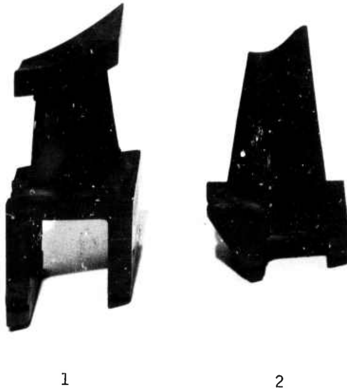
Figure 3.43 — First Stage (1) and Second Stage (2) Design 'B' Stator Segments as Molded
