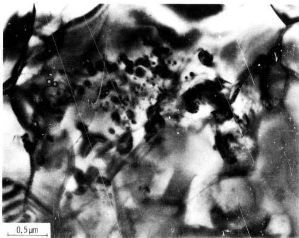
Figure 5.27 — Occasionally observed round impurities with associated strain fields. Also impurity particles in grain boundaries (g.b) 800 kV)
