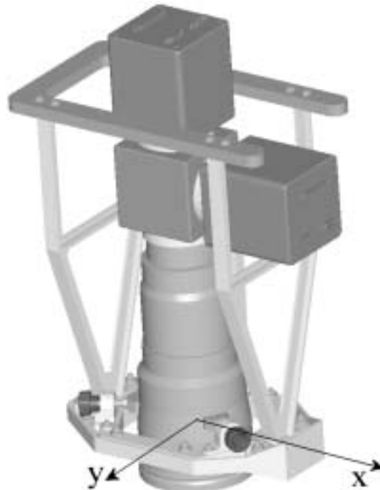
Figure 2. CAD image of camera and absorber with rotation axes.
