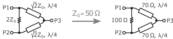
Fig. 16. Schematic of the 3-dB Wilkinson power divider/combiner for an arbitrary system impedance Z_0 (left) as well as for a system impedance of 50\ \Omega (right).
