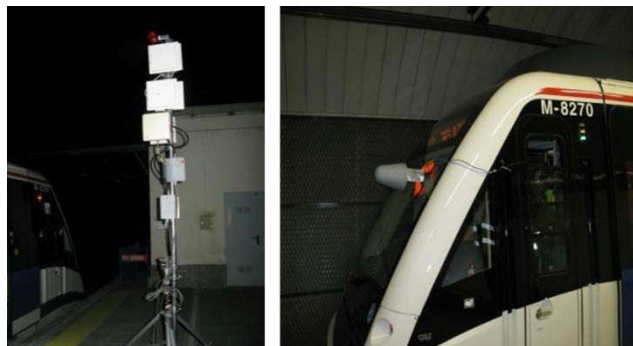
Fig. 7 Radio link measurements on subway tunnels.
