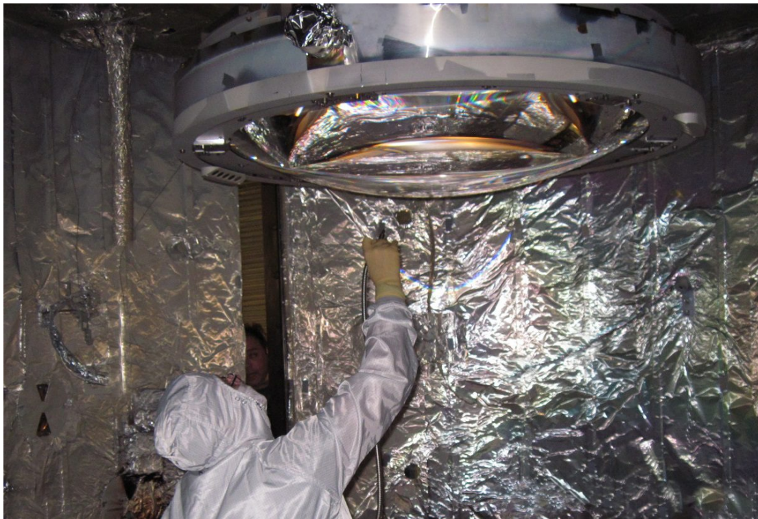
Figure 5. C4 lens in Coating Ring in the chamber at final inspection before starting chamber evacuation.
