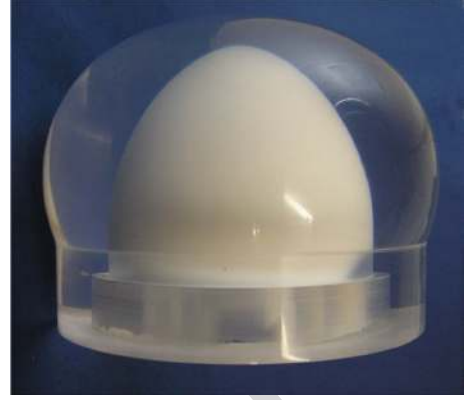
Fig. 4. Fabricated lens prototype with inner shell of MACOR and outer shell of Acrylic.
