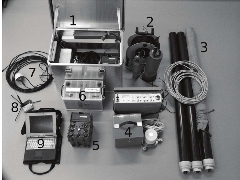
Fig. 2. Components of an AMT-MT instrument in Oulu. 1 = Instrument box containing an interface board, data logger, GSM-modem, regulator for solar panels and battery inside the box and a cable interface outside. The latter has water proof contacts for sensors (nine contacts), external power, GPS antenna, GSM antenna, Ethernet port, USB port. 2 = Pb/PbCl 2 electrodes (five/instrument) and electrode cables (25–100 m), 3 = three induction coils and cables, 4 = three-component fluxgate magnetometer with electronics box and cable, 5 = data logger (EarthData Ltd), 6 = 12V battery (typically 50–120 Ah), 7 = GPS antenna and cable, 8 = GSM antenna and cable and 9 = rugged field laptop.
