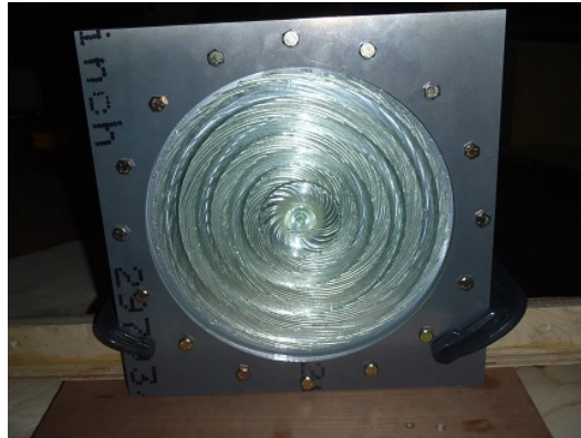
Figure 3.12: Spiral WLS free space optical receiver
