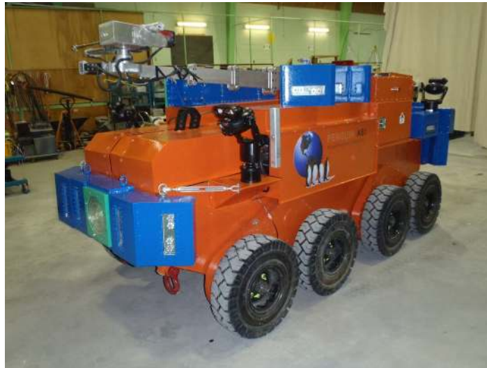
Figure 4.20: Penguin ASI OWC teleoperated demolition robot
