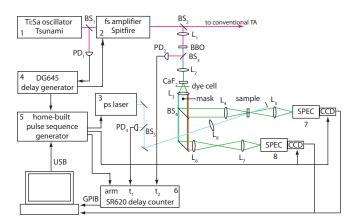
FIG. 1. Schematic drawing of the setup showing only the section with subnanosecond excitation.
