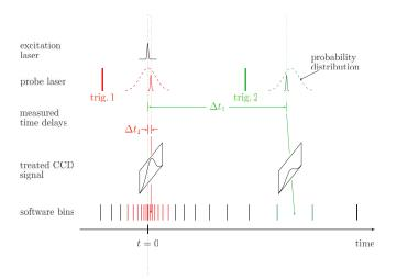
FIG. 2. Timing of the experiment. The two colors correspond to two laser shots with different delay settings.
