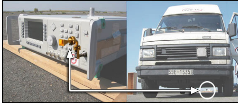
Figure 5. Millimetre wave source and horn antenna as viewed beneath the van.
