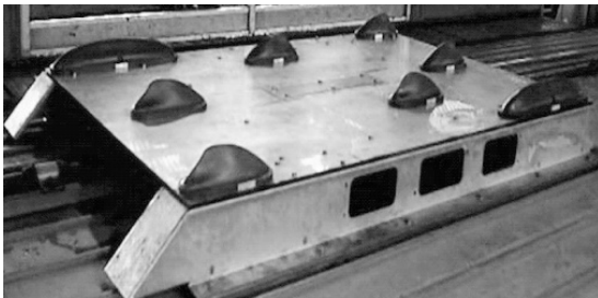
Fig. 6. Antennas on top of the IRIS 320 train.
