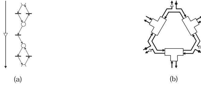
Fig. 16. (a) Ratchet on a line and the corresponding net. (b) Ratchets on the output post-lines of a Brownian TP-Tria. These ratchets will not introduce deadlocks, while the ability to backtrack out of deadlocks inside the TP-Tria is preserved.
