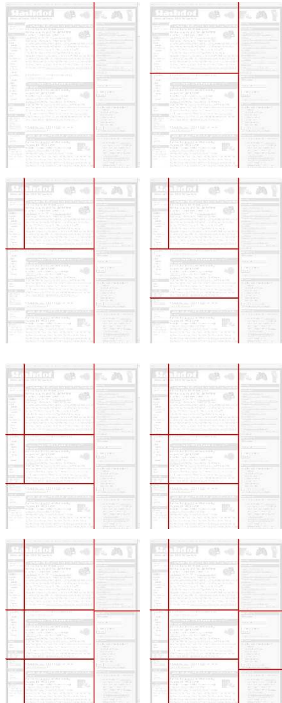
Figure 5. A step-by-step examination of the order in which the Slashdot page is segmented. The order proceeds from left to right and then down. The original image is shown in Figure 4. Note that in this case, all 9 cuts are made. Also note that sometimes images must be cut (the Slashdot logo on top-left) to preserve coherence of the remainder to the page. Final segmentation is on the bottom right.
